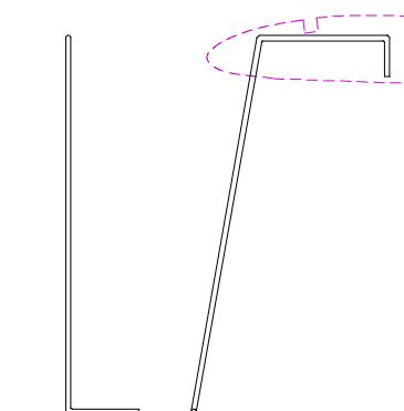
Landing gear from 0.6mm piano wire
